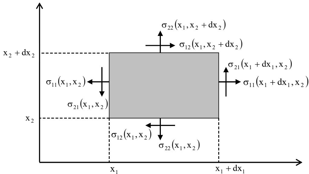
**Exercise 3:** The Cauchy stress field in a solid is given by,  $\sigma_{ij} = \frac{ax_i x_j x_3}{R^5}$  where  $R^2 = x_1^2 + x_2^2 + x_3^2$  and  $a = \text{constant}$ . Examine if there are body forces acting on the body.
